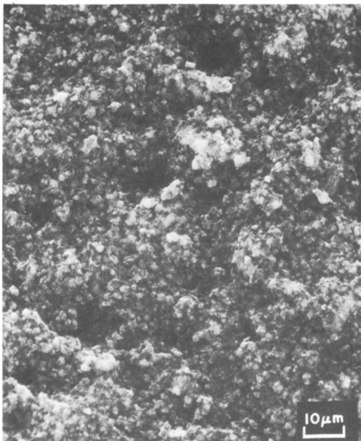
Figure 5 SEM of sample melted in \text{Al}_2\text{O}_3 crucible (leached).
